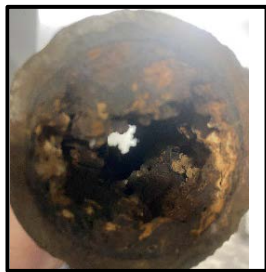
This is a section from the 2-inch main serving several homes.
